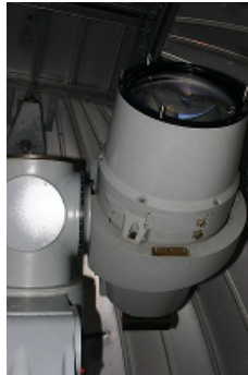
Figure 1.2: Satellite Camera Zeiss BMK75 used in Graz / Lustbühel [20]
