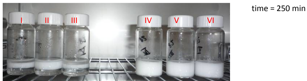
Fig. 21 - emulsion stability test at 80°C; left side, Synperonic L121; right side, Span 80
