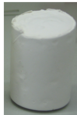
Fig. 16 - COE-monolith after extraction with acetone
