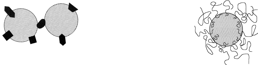
Fig. 3 - steric stabilization of emulsion droplets - left: solid particles; right: polymers (reprinted from ref 12)
