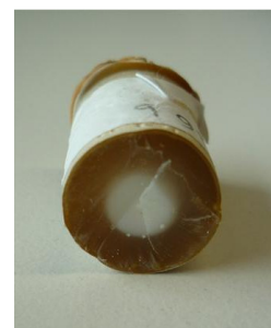
Fig. 35 - “core-shell” structure of collapsed monoliths (sample 76b, 50:50 copolymer)
