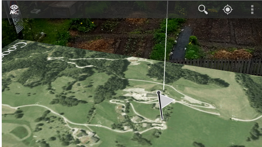
Figure 5.5: AR browser exploration example: a white line connects the POI annotation and the position on the overview map. This helps to find the place on the map, which is annotated with the gray flag marker.
