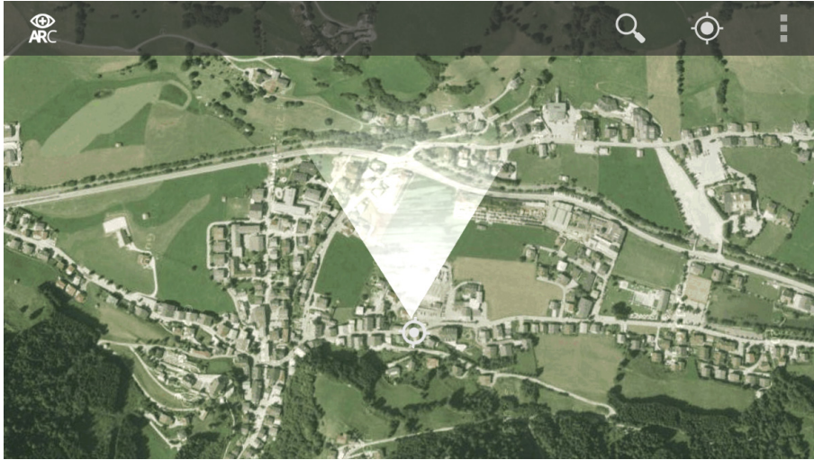
Figure 5.2: AR browser exploration example: pointing the device on the ground to show the map. Only the FOV indicator is shown and nothing is highlighted by markers.
