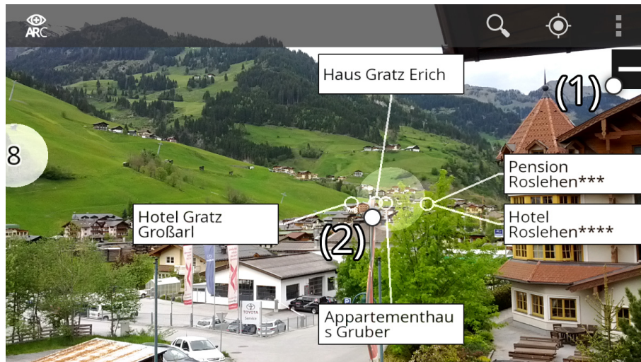
Figure 5.7: AR browser exploration example: the visualization of the cluster after clicking on the plus-icon of Fig. 5.4. A tap on the minus-sign (1) allows to return to the previous level and touching the area at (2) exits the cluster data detail visualization.
