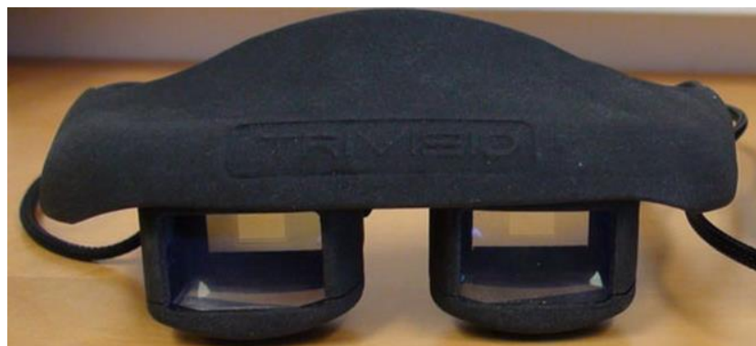
Figure 14: The OLED based binocular interactive see-through HMD Eval-Kit (Fraunhofer Research Institution for Organics, 2014)
