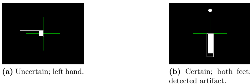
Figure 5.3: Visualization of the way how feedback was provided. A white frame indicates the target class. The fraction of the classifier's output probability for the target exceeding 0.5 was displayed as a white bar. A white dot above the green fixation cross tells the participant that an artifact was detected.
