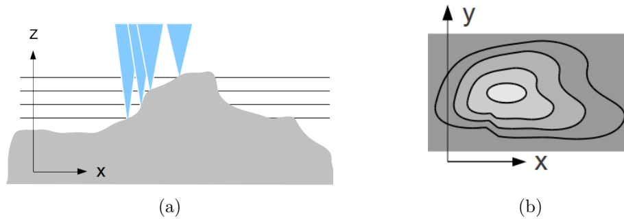
Figure 3.15: (a) Alicona principle: Determination of the topography data by focus variation and (b) 2D map of the surface, denoted by contour lines
