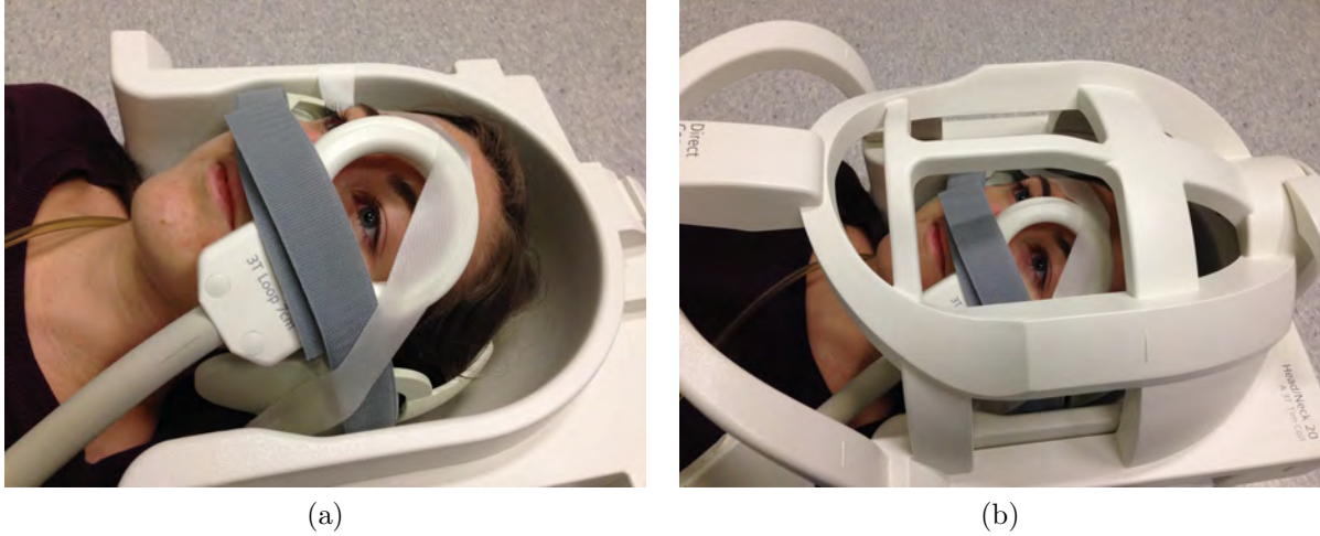
Figure 3.1: For in vivo SNR measurements the small surface coil was placed over the left eye and fixated with a velcro strip and medical tape (a). Sequences were measured with three different coil settings: only head coil, only loop coil and both in combination (b).
