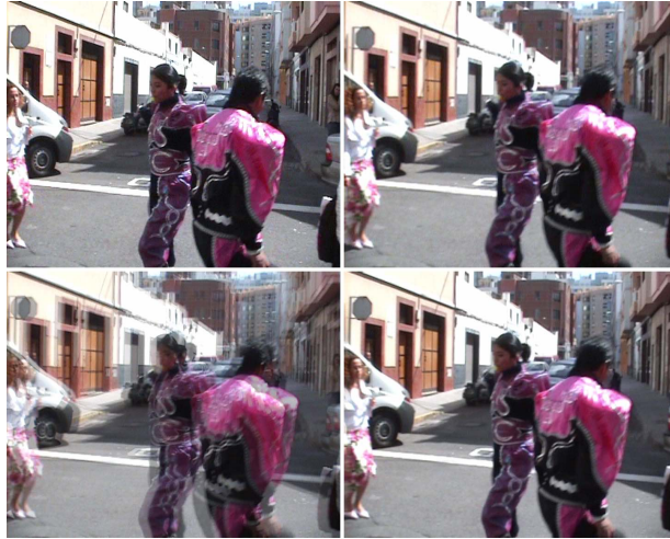
FIGURE 1.4: Comparison of the simple frame blending approach and the forward frame interpolation approach. The upper row shows the two consecutive input images of the frame interpolation algorithm. In the lower left, the visually poor result of the frame blending approach is visible. The lower right image shows the interpolated result of the frame interpolation algorithm, proposed by Dudek et al. [17]. The images are taken from [17].
