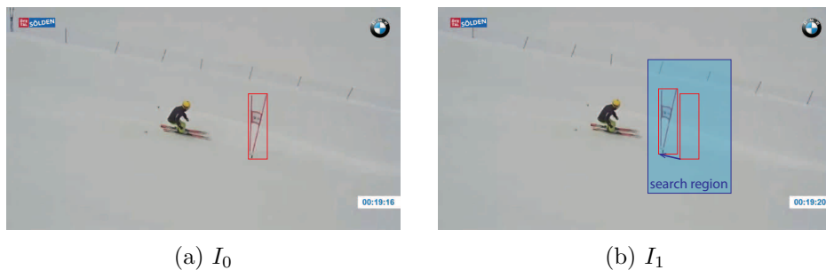
FIGURE 3.24: By using a limited search region for the sliding window approach instead of the whole image, the computational expense can be reduced. Furthermore also the likelihood for false matches is decreased, because less candidates are considered in the matching process.
