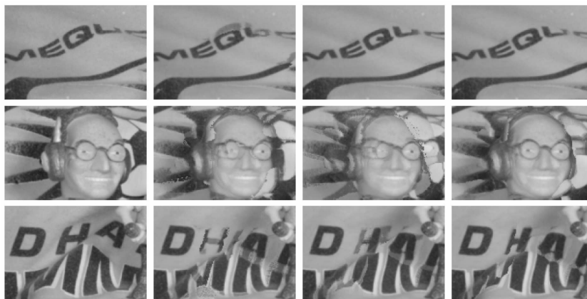
FIGURE 1.6: Comparison of different frame interpolation approaches. From left to right column: ground truth images, forward interpolation, backward interpolation, symmetrical approach by Rakêt et al. [31]. It can be observed, that the symmetrical approach yields a visually good result, with less artifacts in comparison to the other two approaches. The images are taken from [31].
