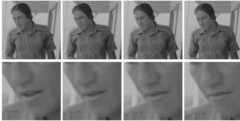
FIGURE 1.5: The leftmost and rightmost column contain the input images and the center columns the interpolated images. As can be seen in the enlarged frames in the bottom row, the bidirectional frame interpolation algorithm of Werlberger et al. [42] yields visually attractive results. The head movement and the mouth closing are interpolated without visible artifacts. Furthermore, also the occluded region in the background is handled correctly. The shown images are taken from [42].
