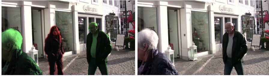
FIGURE 3.19: The video inpainting algorithm of Granados et al. [20] yields visually pleasing results, even for complex background scenes. A mask for objects to be removed and a mask for dynamic objects which remain in the image is required. The images are taken from [20].
