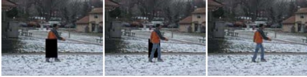
FIGURE 3.17: The video inpainting algorithm of Patwardhan et al. [29] takes spatial and temporal information into account to fill the target region. The method is limited to image sequences with a stationary camera. These images are taken from [29].
