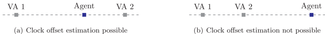
Figure 3.3: Case study: Estimation of the clock offset. In (a) a scenario is shown, where perfect clock estimation is possible when having equal SINRs from both VAs, although localization is not possible. On the other hand in (b) the estimation of the clock offset is not possible when not having prior knowledge about the agent position.
