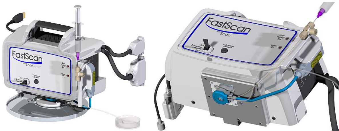
Figure 22: FastScan Bio hardware with micro-volume fluid cell mounted for biological AFM experiment front view (left) and from below (right) [50].
