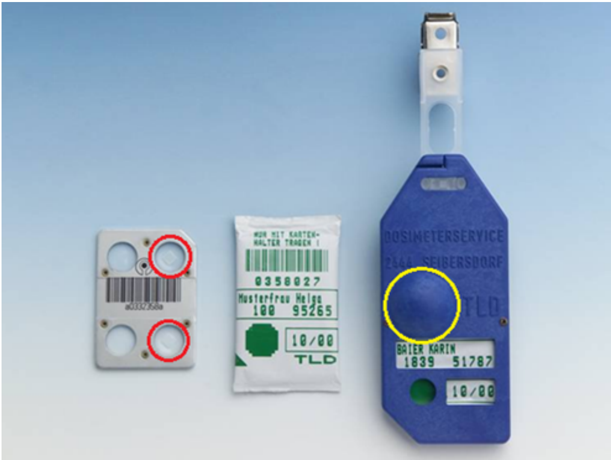
Figure 4.1.: On the left side a TLD-100 card is shown containing two chips of \text{LiF:Mg,Ti} at card positions 2 and 3 (red circles). This card is then sealed and provided to the customer (in the centre). On the right side the card is shown as placed in the card holder. One of the two elements is shielded with a thin aluminium disc (yellow circle). This allows to apply different weights for hard and soft radiation.
