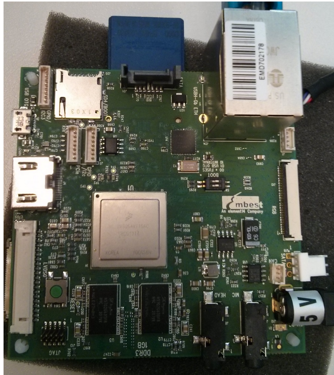
Figure 4.2: Evaluation kit for the Freescale i.MX6Q processor
