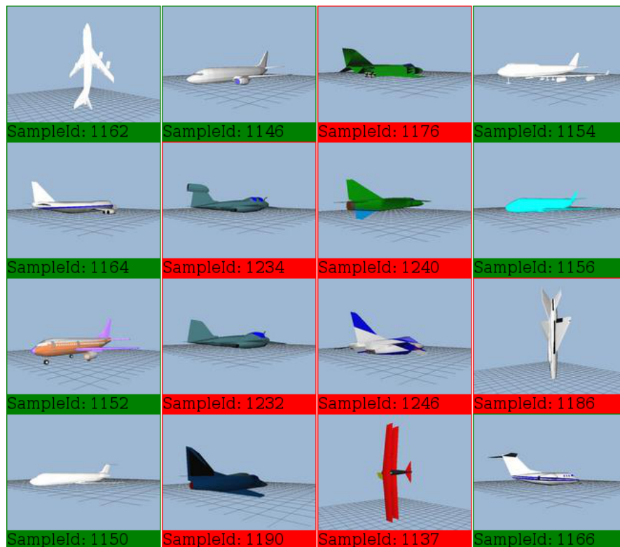
FIGURE 5.5: The top 16 retrieval results for the class commercial airplane. Even though all models in the top results are airplanes, there are many false positives. That is because the Princeton benchmark distinguishes between many different airplane classes (commercial, fighter, biplane etc.), and we only search for commercial airplanes.
