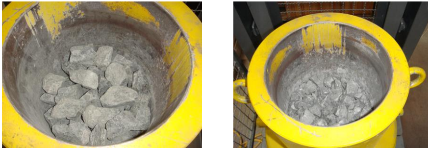
Figure 8: sample in mortar before (left) and after impact test (right), the sample is adjusted in the mortar by hand, before the test.
