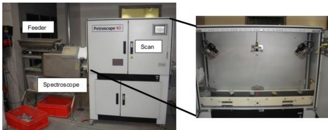
Figure 10: overview of the device Petroscope 4D ® (left) with the feeder, spectroscope and scan unit; inside the scan unit (right) with the conveyer belt, laser and cameras.
