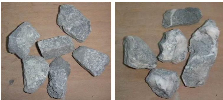
Figure 14: Example for one of the separation criteria, Diabase “A” and “B” with and without quartz lenses/veins
