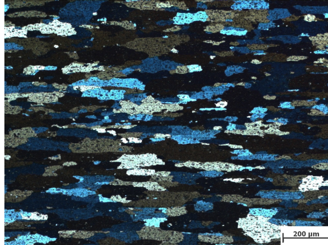
Figure 79: LOM of a sample cold rolled and annealed for 10 minutes at 350°C
