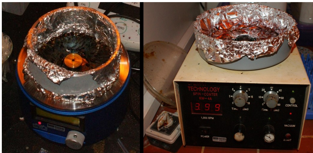
Figure 2.4.: The different spin-coaters used. The right image shows a KW-4A spin-coater placed in the fume hood. The image on the left shows a K.L.M. SCC-200 spin-coater inside the glove box.
