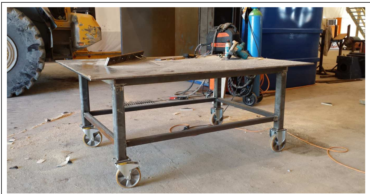
Figure 38: Produced movable working table
