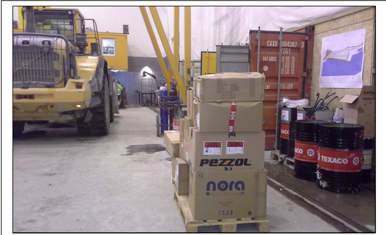
Figure 4: Incoming goods blocking the rail of the portal crane
