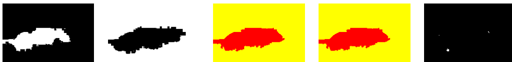
Figure 16: Iteration 3: Updated unary potentials for semantic classes 'rhino/hippo' and 'water', segmentation before and after graph cuts regularization, and difference between segmentations (24 pixels) (left to right).
