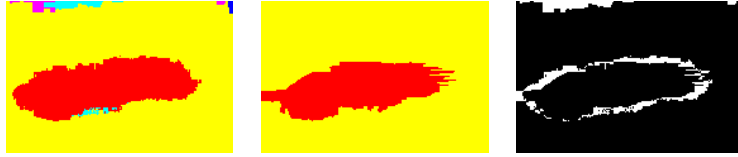
Figure 14: Iteration 1: Segmentation before (left) and after (middle) graph cuts regularization and difference between segmentations (1537 pixels).
