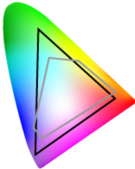
Figure 2.2: CIE XYZ Chromaticity Space compared with sRGB (black) and CMYK (gray). Image taken from http://www.posterlia.at/service/softproof.html
