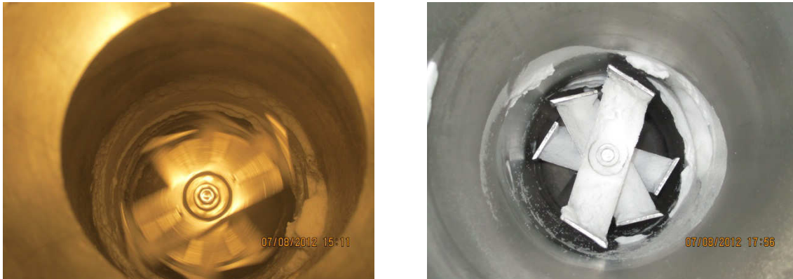
Figure 5-29: Left: Start-up phase. Material stuck to the wall. Right: Process end, little material residues are found.
