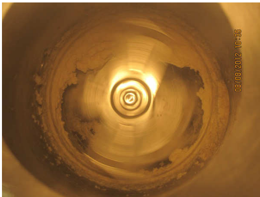
Figure 5-39: Start-up phase for flour slurry. The lower dryer chamber is filled by dough.
