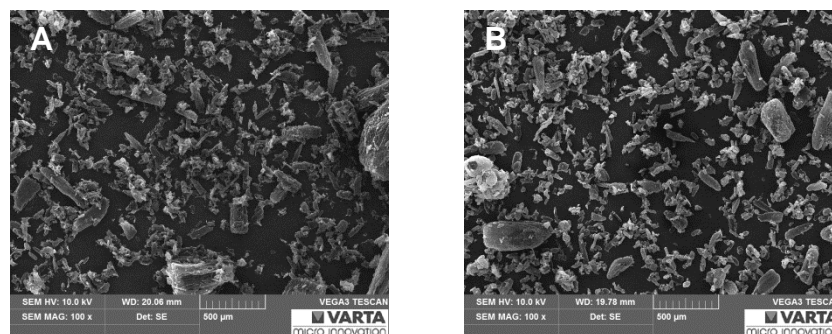
Figure 5-31: SEM image of benzoic acid at a magnitude of 500. (A) feed and (B) SFD 67.
