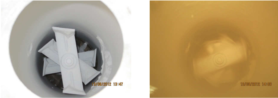
Figure 5-33: Salicylic acid particles covering dryer wall (left). Particles being blown off (right).
