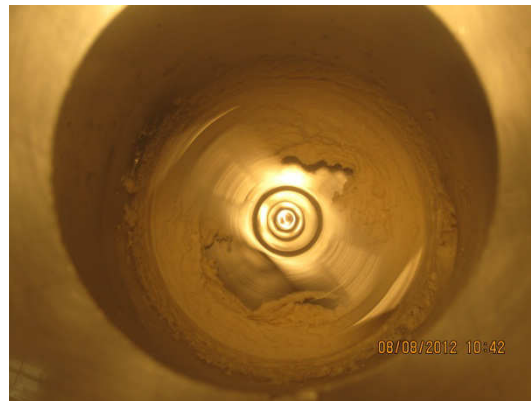
Figure 5-39: Start-up phase for flour slurry. The lower dryer chamber is filled by dough.
