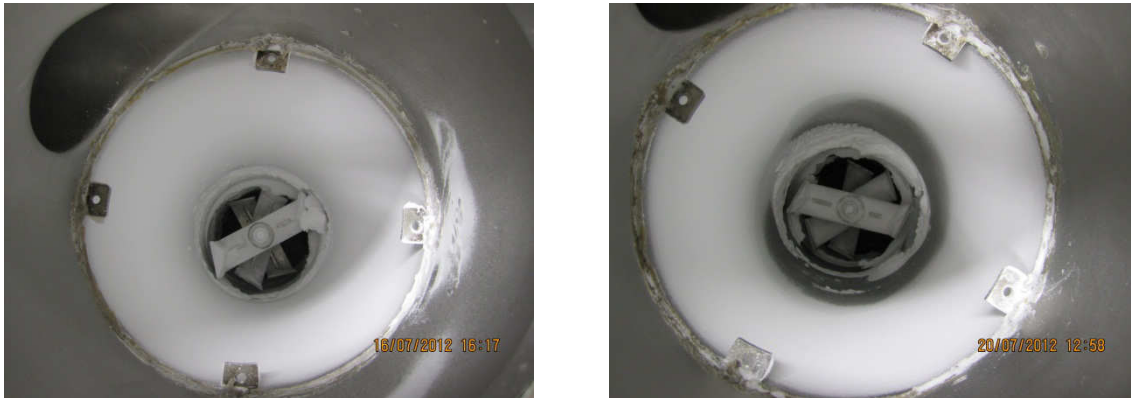
Figure 5-2: Adipic acid DoE experiment with dry particles adhering on the dryer wall.
