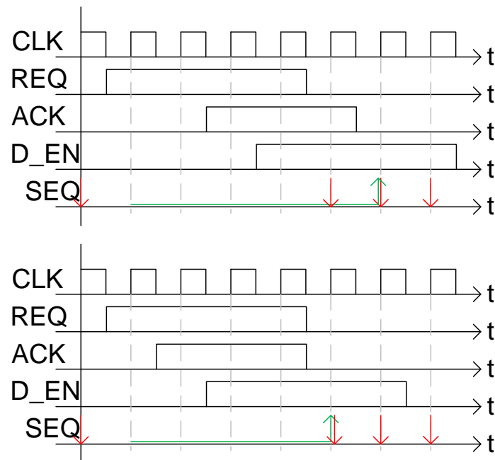
Figure 2.12: An example of a typical handshake protocol, two different ways that would both be valid for the defined sequence (there are more valid possibilities), green lines show where the sequence is running, a green arrow where the sequence is successfully finished and red arrows where a sequence checking run is stopped due to a mismatch
