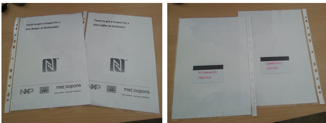
Figure 5.4.: Smart posters for two issuing tags based on JCOP contactless smart cards (left). The tags have been attached on the back, right behind the NFC logo to indicate the touch point (right).
