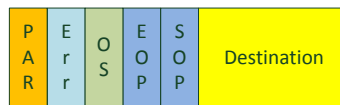
Figure 5.5: New packet containing information about the parity in the „PAR“ field of the packet.
