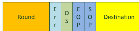
Figure 5.4: New packet containing information about the round in the „Round“ field of the packet.
