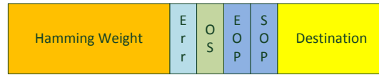
Figure 5.6: New packet containing information about the parity in the „Hamming Weight“ field of the packet.
