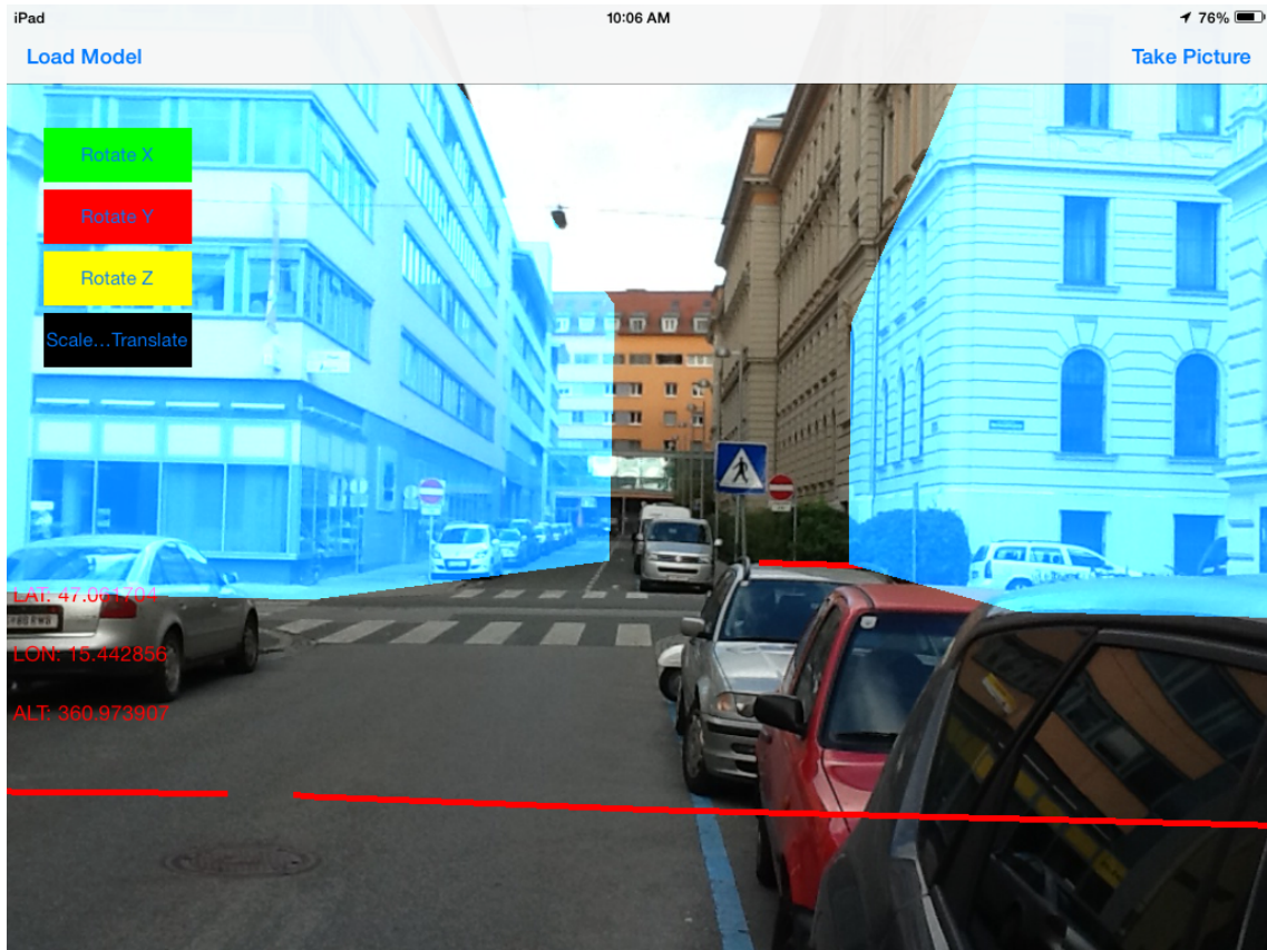
Figure 4.6: Screenshot of the prototype shows the correction tools, Rotate X , Rotate Y , Rotate Z , and Scale or Translate .
