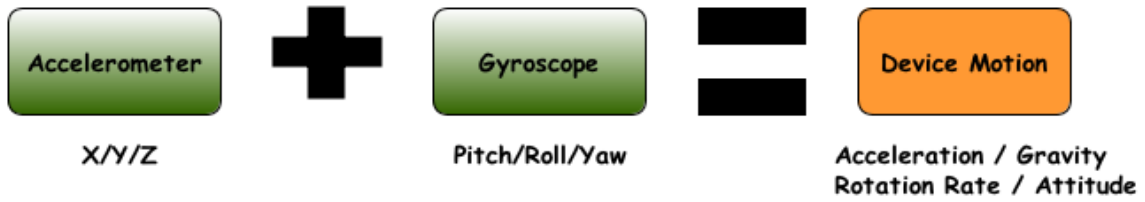
Figure 3.2: Combining the Accelerometer's data with the data from Gyroscope to get the Device Motion.
