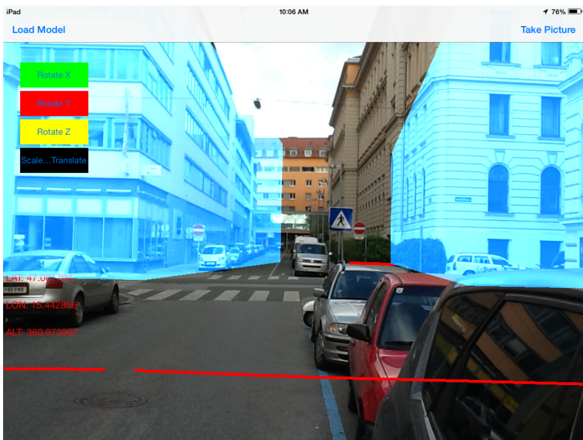
Figure 4.2: A screenshot of the prototype, two buttons on the top bar, Take Picture and Load Model are for taking the picture of the real world and loading the virtual model respectively. On the other hand the colored buttons are used for the correction method. And the red labels report the current latitude, longitude, and height.
