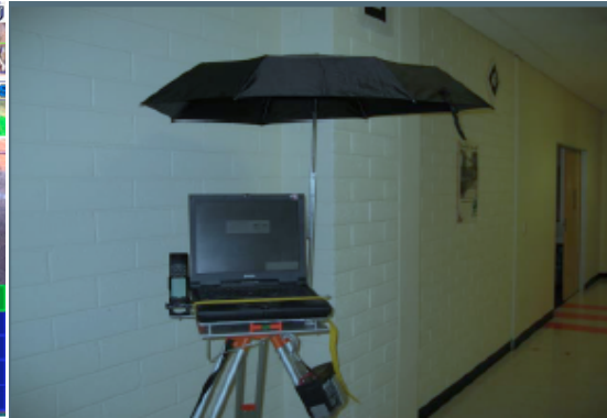
Figure 2.10: ARVino hardware with laptop, tripod, and umbrella [15].
