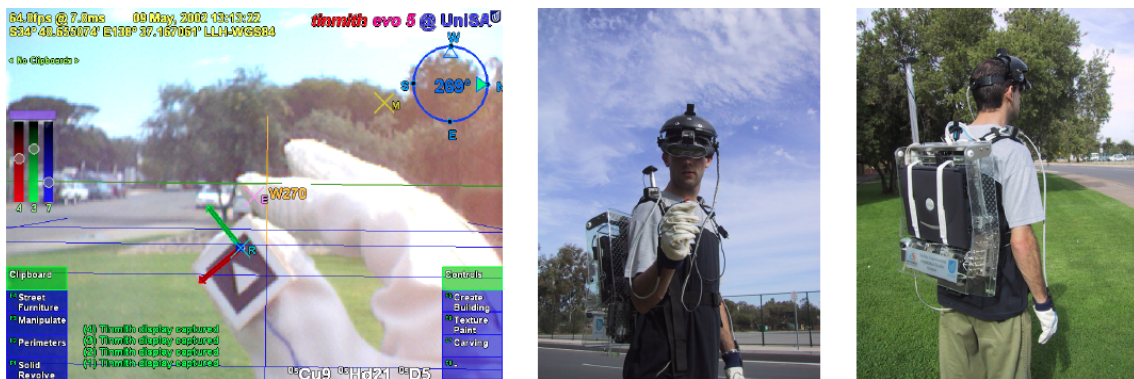
Figure 2.11: Mobile Outdoor Augmented Reality Modeling Demonstration. The picture to the left shows Modeling cursors with pinch gloves, in the middle is a front view of the backpack and the head-worn display, and to the right is a rear view [18].
