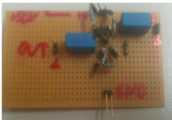
Figure 3-12: Signal amplifier circuit (left) and schematic of the circuit (right)
