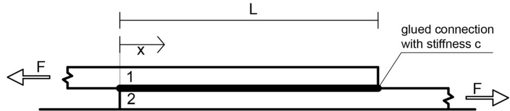
Figure 42: Shear connection with an elastic layer between the members
