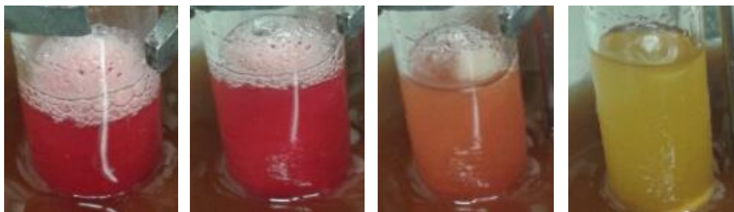
Figure 3: colour change and nitrogen evaporation during an iEDDA
