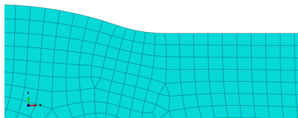
Fig 5-1 The current mesh generation with 5 equal size linear elements at the surface. Inverse Y-joint. The notch is located at toe 2.
