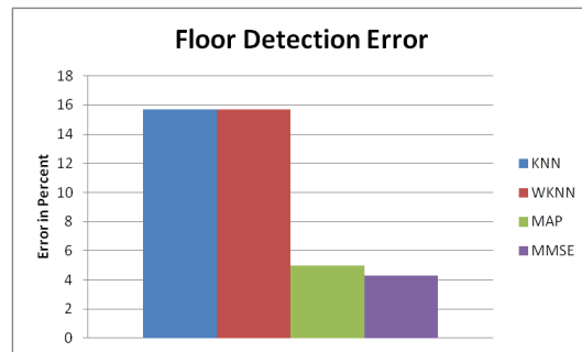
Figure 4.15: Floor detection error by using the same number of training samples at each floor.
