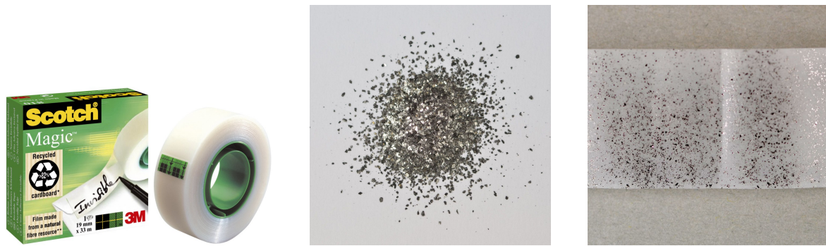
Figure 3.1: The used adhesive tape type (left), raw natural graphite flakes (middle) and thinned graphite sheets on the tape (right)
