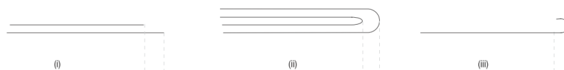
Figure 4.16: Three ways how a double line at a graphene edge can be composed of: i) staggered edges of bilayer graphene, ii) bilayer completely folded back, iii) SLG forming a nanotube on the edge (from [136])
