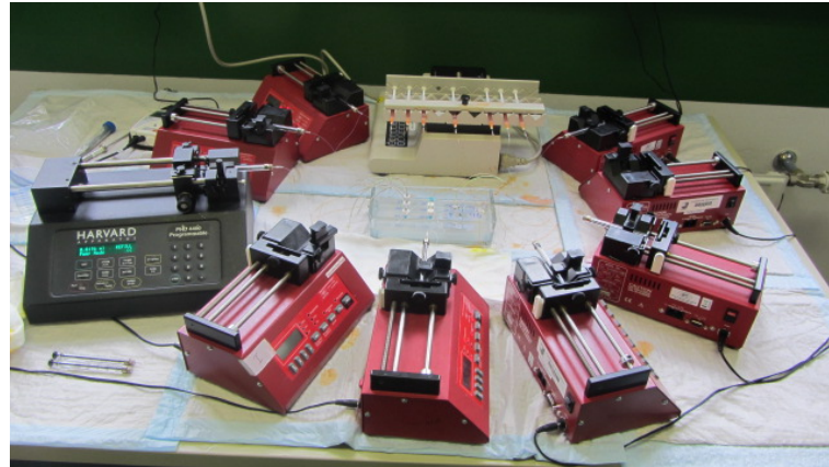
Figure 2.16.: Measurement setup of the in-vitro feasibility studies. The 8 pulling AL-ADDIN syringe pumps (red), the pulling HARVARD pump (black) and the pushing 10-channel syringe pump (white) surround the laboratory dish with gel network, matrix plate and probe types.
