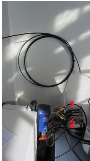
Fig.2. Before starting the measurements, make sure that both air exits of the compressor are connected with the rheometer.
