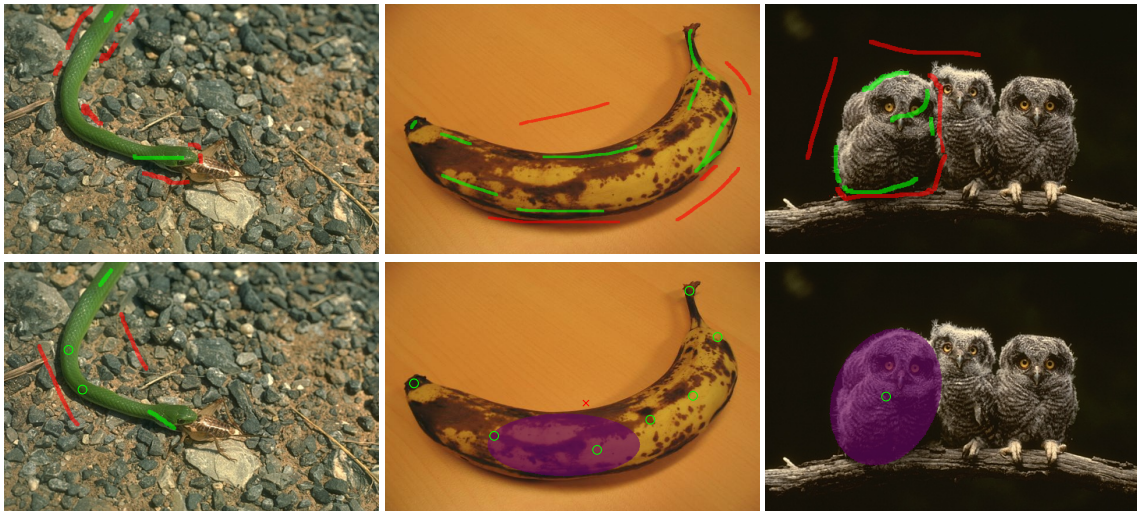
Figure 5.15: The shape constraints as well as the weighting map are obtained from a single user-specified ellipse illustrated in (a). Segmenting a single owl out of a group of owls is achieved by using covariance, area and star prior constraint. The star center equals the CoG of the ellipse and is denoted by a green circle in (a).
