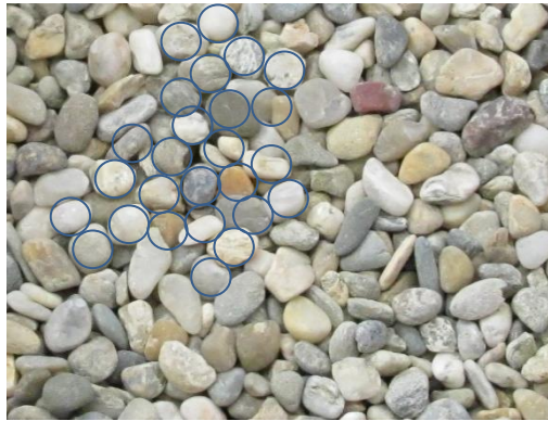
Figure 16: Discretization of the pea gravel
