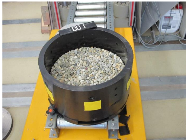
Figure 23: Oedometer test on pea gravel
