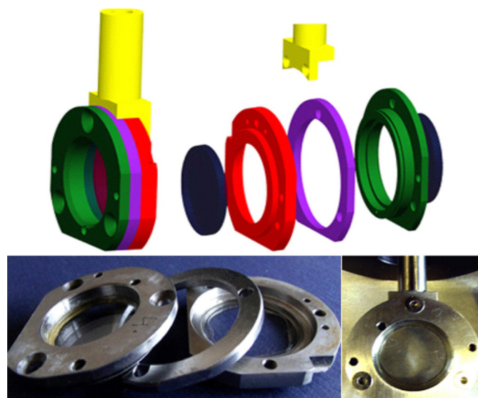
Fig. 2. Flat sample-cell. Top: schematic view. The cell consists of two main parts (red and green) with glued-in glass windows (optical flats, dark blue) and o-ring sealing. The sample thickness is controlled by the middle spacer ring (pink). The cell is connected to the stepper motor by the yellow shaft. Bottom left: section view; bottom right: front view, assembled.
