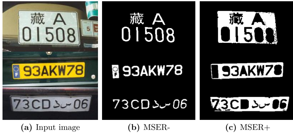
Figure 2.1: License plate detection using MSER . (a) Input image with various license plates from different countries. (b) The individual characters of the plates detected using MSER - regions. (c) The license plates detected as a MSER + region. (Images taken from [16])
