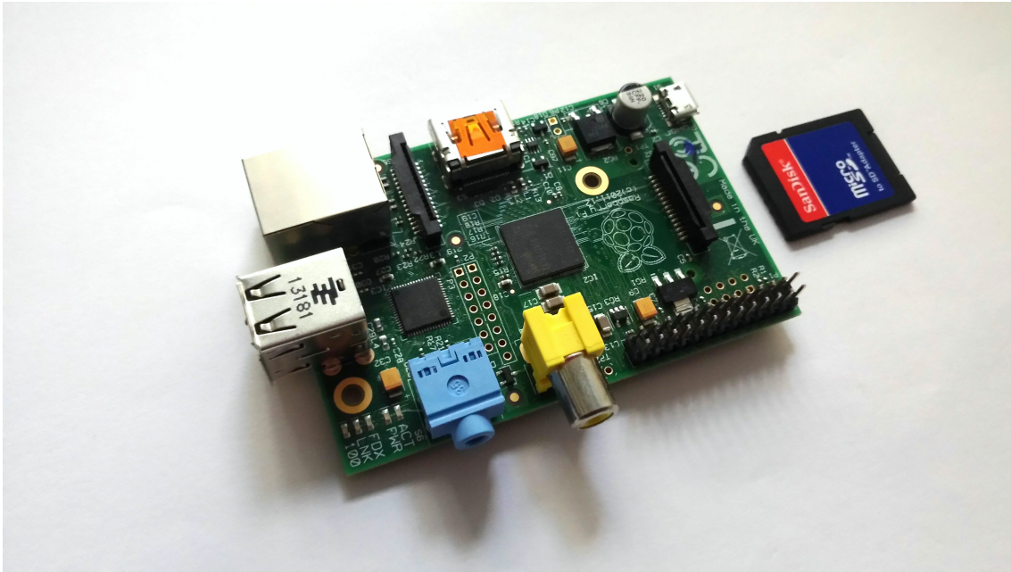
Figure 4.3: The figure shows the Raspberry Pi Model B, with the used SD card
