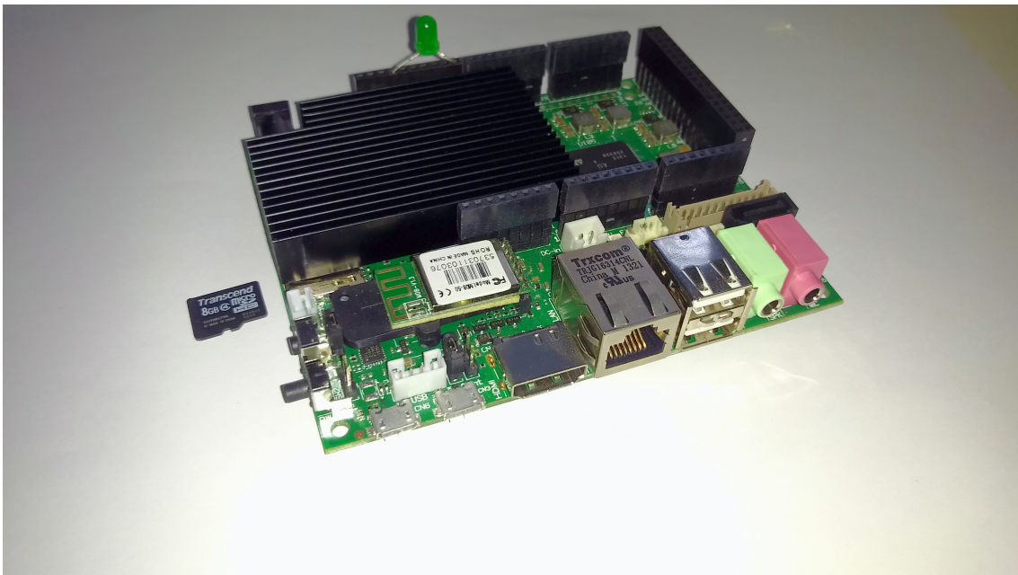
Figure 4.4: The figure illustrates the UDOO quad ARM board and the used micro SD card.
