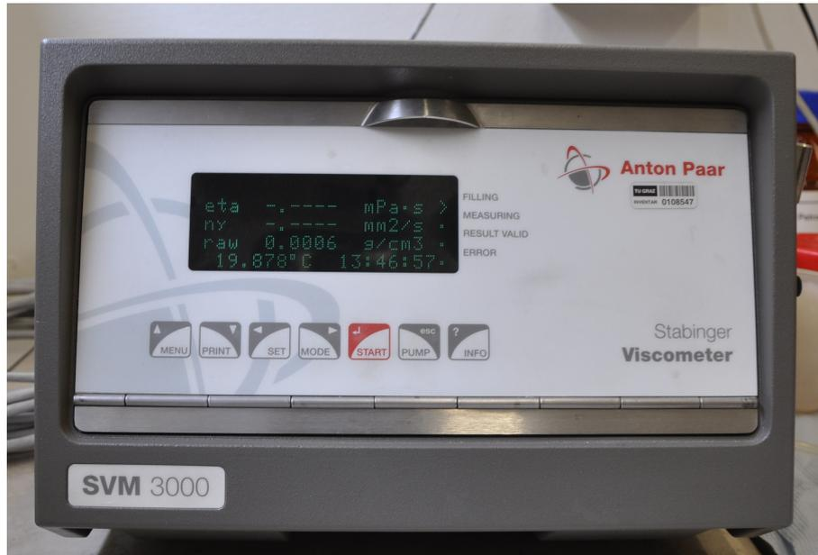
Figure 3.15.: Photo of the viscometer
