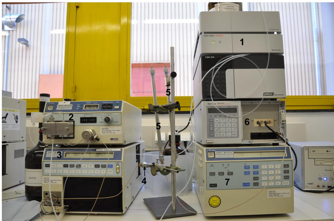
Figure 3.13.: GPC system with precolumn and two separation columns
