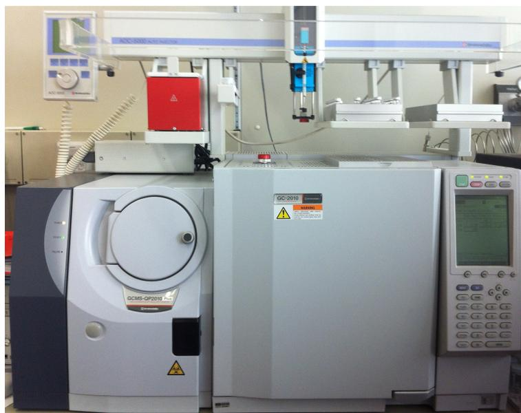
Figure 3.11.: Photo of the GC-MS system
