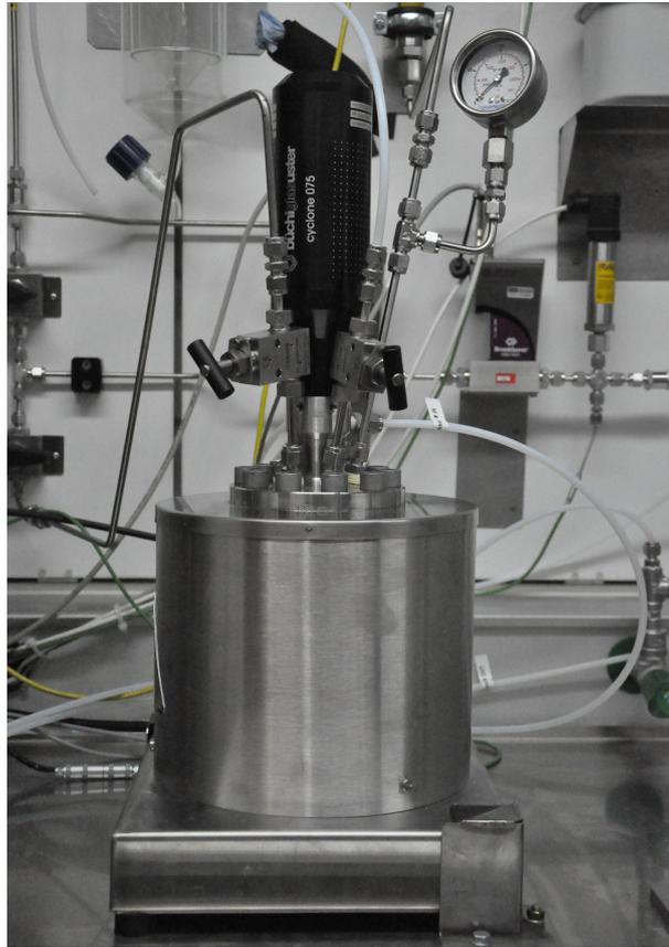
Figure 3.5.: Photo of the HDO reactor
