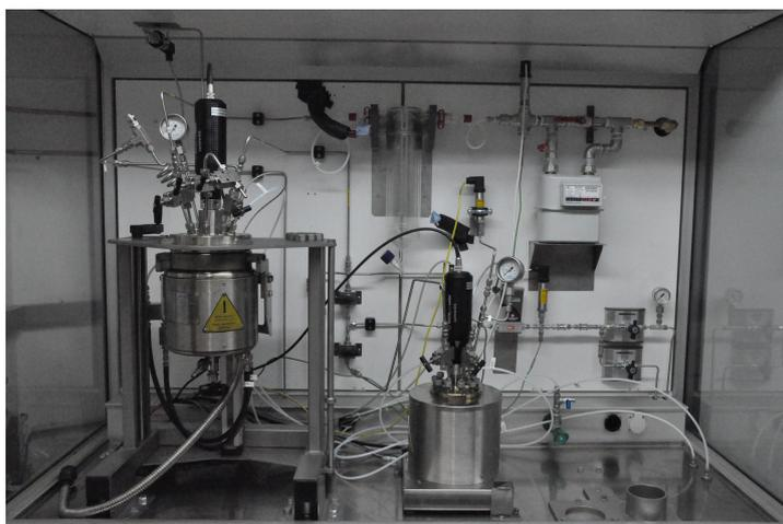
Figure 3.4.: Photo of the whole set-up of the HDO reactors, reactor II is the reactor on the right
