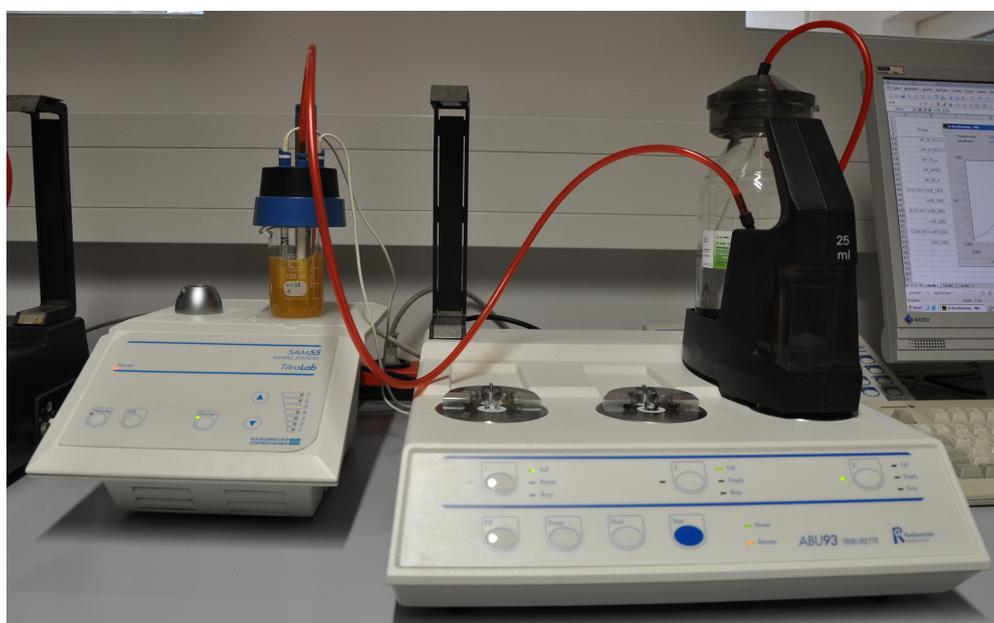
Figure 3.16.: Photo of the autotitration system
