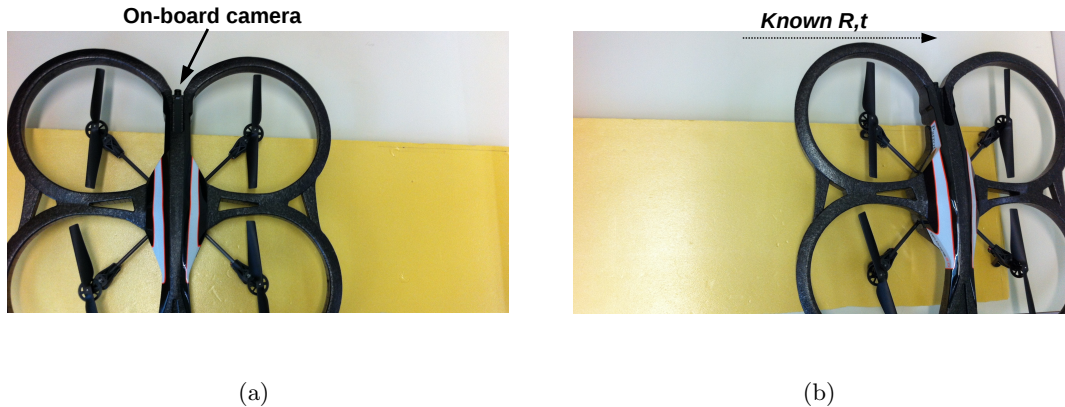
Figure 3.3: Metric PTAM initialization. (a) The UAV is placed on the left marked position from where the first keyframe is captured. (b) The second keyframe is captured from the right position, which is also marked on the board. The relative motion between the keyframes is known in terms of \mathbf{R} and \mathbf{t} , which results in a metrically scaled initial map.
