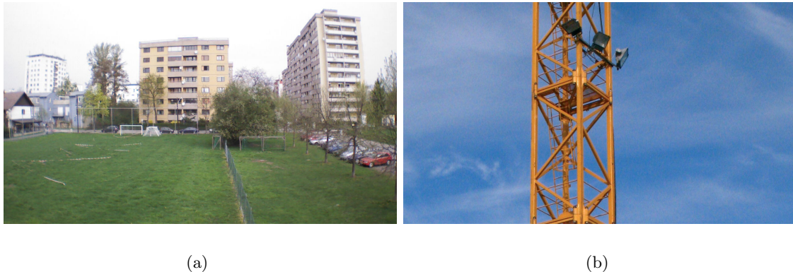
Figure 3.5: Some situations showing the limited feasibility of PTAM on unmanned aerial vehicles. (a) Large scenes cannot be mapped accurately due to small triangulation angles. (b) Lack of texture or missing map points in the field of view cause PTAM to lose localization .
