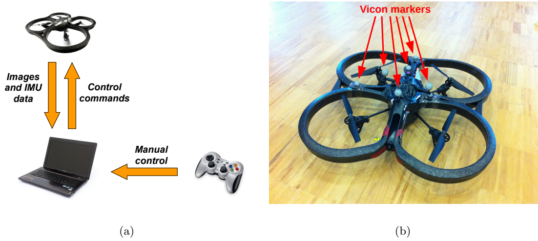
Figure 6.1: Experimental setup. (a) The AR.Drone 2.0 communicates with the ground station laptop over a Wi-Fi link. For manual control we utilize a gamepad to communicate with the drone via the ground station. (b) Special markers on the drone allow highly accurate 6DOF pose estimates using the Vicon motion tracking system.
