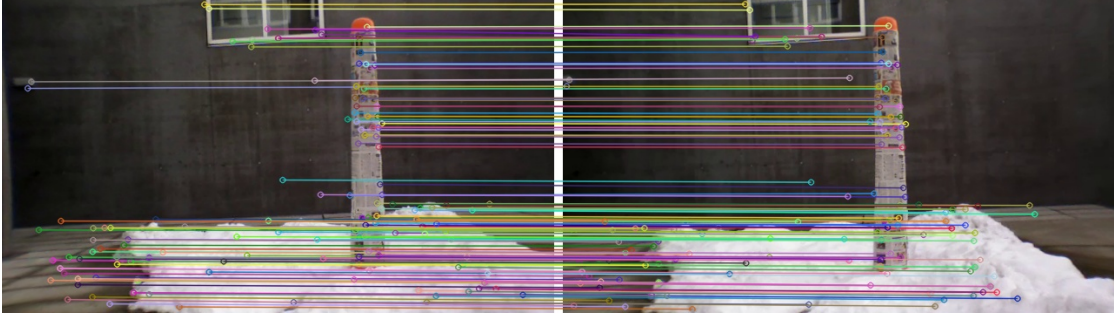
Figure 4.7: Using a ratio matcher with backmatching leads to high quality correspondences. We used a distance ratio threshold T_{ratio} of 0.7.
