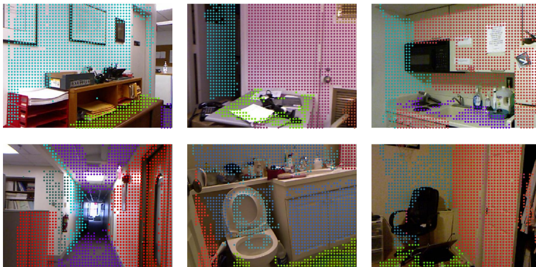
Figure 5.5: Examples of RGB images of the NYU depth dataset with planes constructed from planar regions (walls, ceilings, floors) in the depth data.
