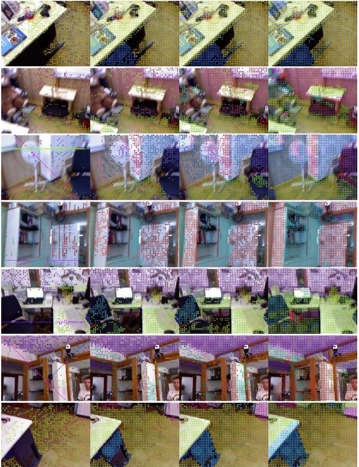
Figure 5.2: Testing different inlier thresholds with Sequential RANSAC (4 iterations). From left to right: \tau = 0.001, 0.005, 0.01, 0.05 . The threshold in the leftmost column is too sharp to detect all relevant planes, and it introduces artifacts: when a hypothesis is constructed from a subset of which the image coordinates are collinear, then it forms a plane perpendicular to the camera. With a very low inlier threshold, these planes score higher than others, because a number of points is guaranteed to lie on the plane, and they are thus selected by the RANSAC algorithm. \tau = 0.05 is too imprecise, as we can see in the bottom right image, where a part of the desk surface is labeled incorrectly. \tau = 0.005 and \tau = 0.01 (center columns) both seem to be legitimate choices.
