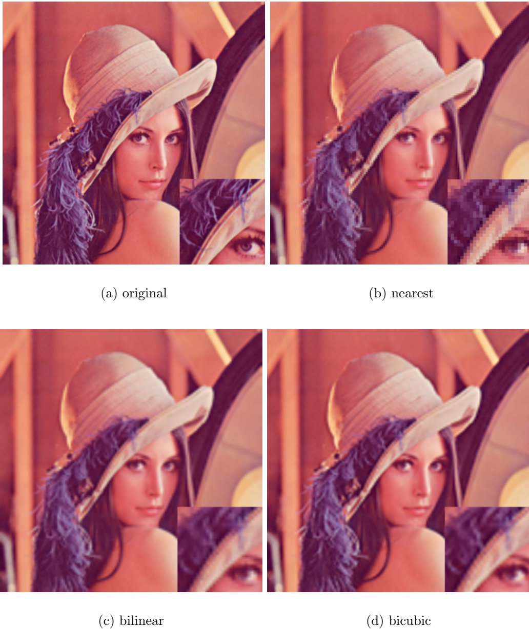
Figure 2.2.: Result of basic image interpolation algorithms upsampled by a magnification factor of 3. First image shows the original input file of size 254 x 254 pixels. The following images from left to right show interpolation results of nearest-neighbor (29.1dB), bilinear (30.1dB) and bicubic(31.4dB) interpolation respectively.
