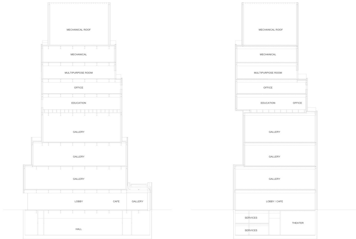
Figure 5-19 - Section through the Building
