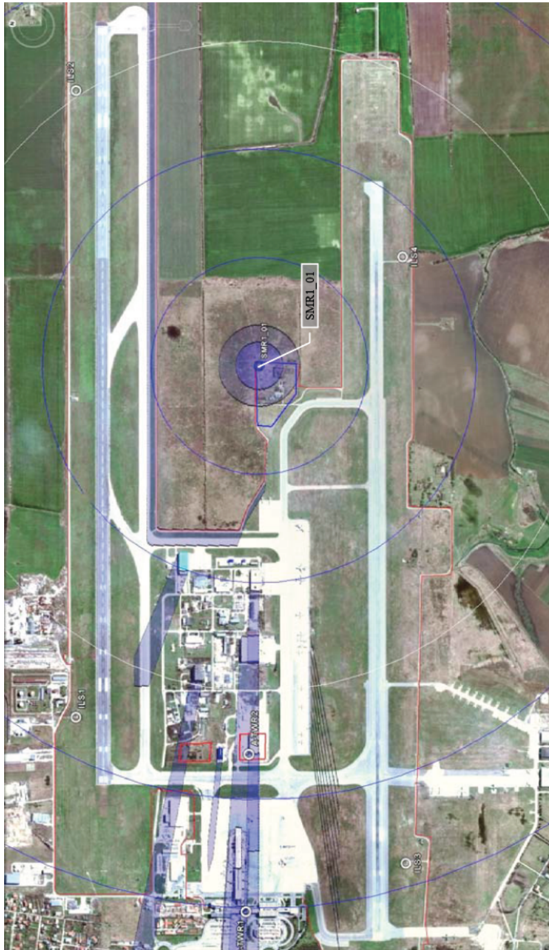
Figure B.3.: Visualization of areas without radar coverage due to "shadowing" for SMR-East at Bucharest Airport (in dark blue)
