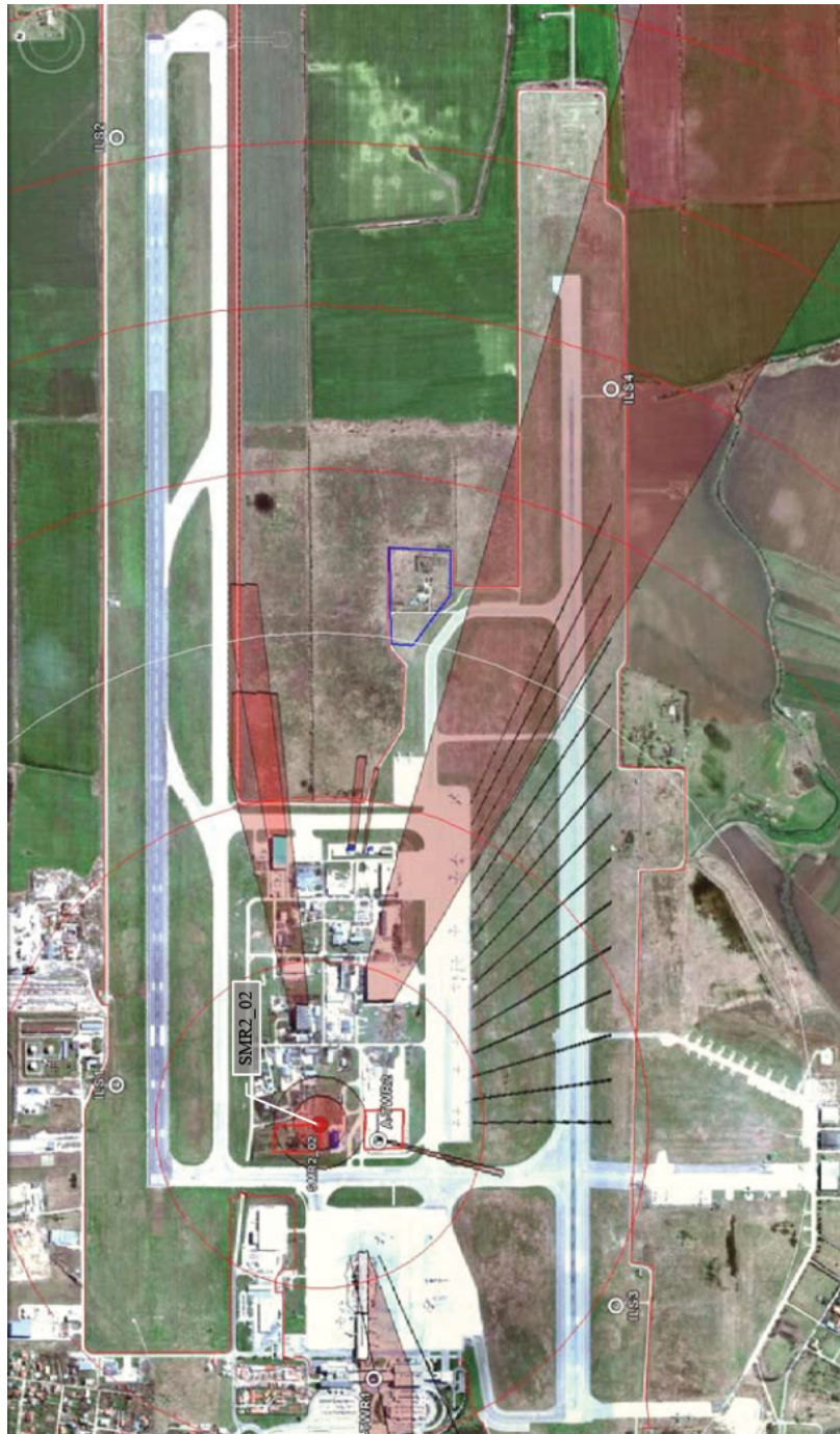
Figure B.2.: Visualization of areas without radar coverage due to “shadowing” for SMR-West at Bucharest Airport (in red)
