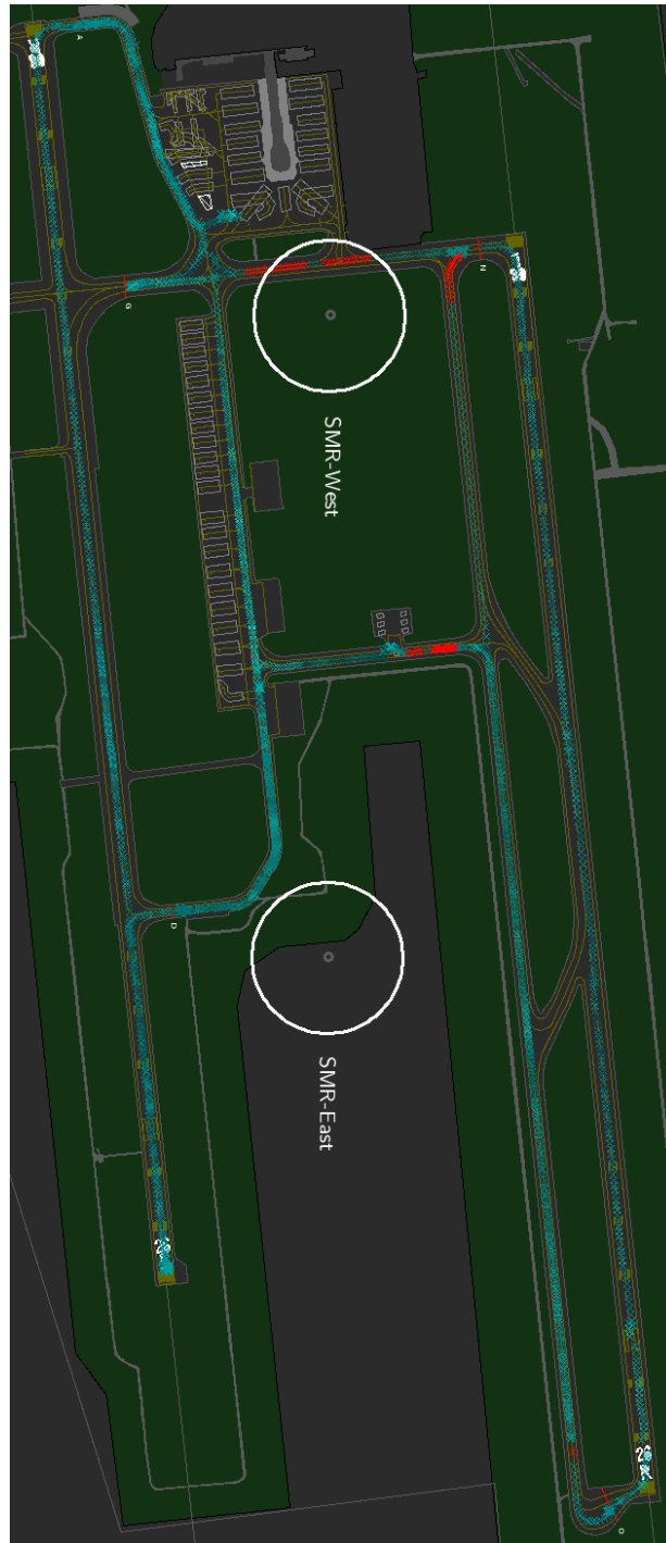
Figure 4.5.: Visualization of probability of detection analysis results (Both Radars, Tracked). Blue crosses are target detections, red crosses are missed target detection. Deadcones of radars visualized as white circles
