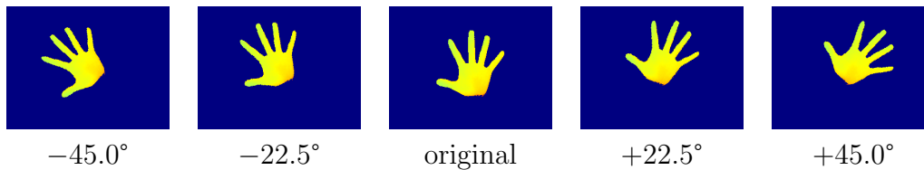
Figure 26: Rotated depth images. Each captured depth image (figure in the mid) can be additionally in-plane rotated so that several rotations are covered as shown on the left/right side. The complete dataset also contains further rotated images ( \pm 67.5^\circ , \pm 90.0^\circ , \pm 112.5^\circ , \pm 135.0^\circ , \pm 157.5^\circ and 180.0^\circ ).
