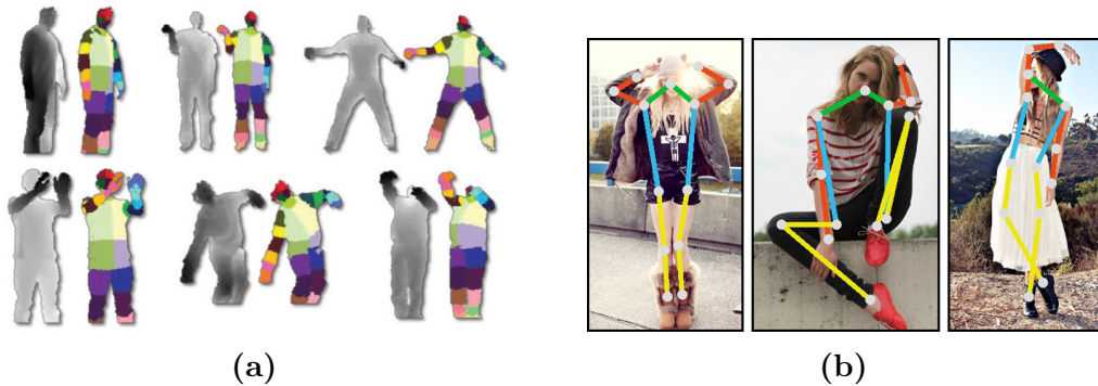
Figure 5: Body pose estimation. The example images are taken from [45] and [11], respectively. Again, we show depth and color images where (a) performs a per-pixel classification of different body parts and (b) formulates a regression problem to predict the coordinate of several joint locations of the body.
