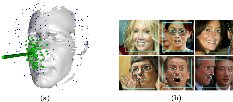
Figure 4: Head pose estimation. The example images are taken from [13] and [10], respectively. Both approaches estimate the direction to which a head points but (a) estimates the nose position as well as its orientation on depth image patches and (b) estimates the label of the head orientation and then several facial feature points, done on color images.
