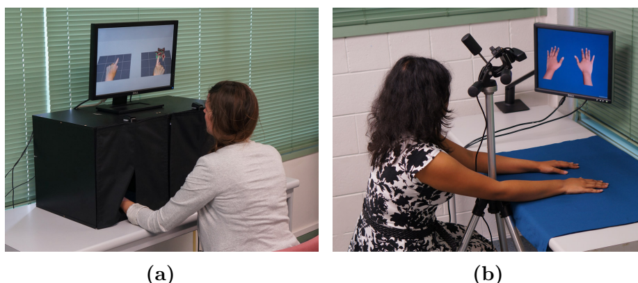
Figure 1: Setup of the ART system for post-stroke rehabilitation. We have adapted the current system where (a) the prototype consists of boxes to provide a controlled environment. The proposed system is (b) a free table solution with a colored fabric as background so that the hand in the foreground can be easily segmented.
