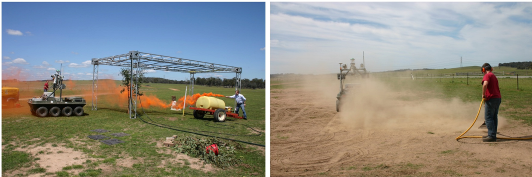
Figure 2.3: Static (left) and dynamic (right) test area for camera and laser scanners [3].
