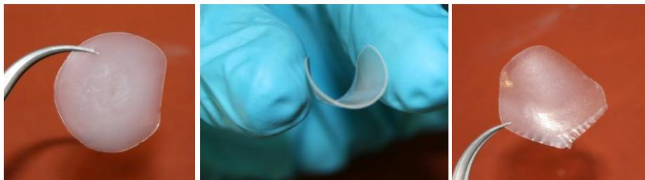
Fig. 25: Cellulose substrates; primary gel (left and middle) and FSEC (right).
