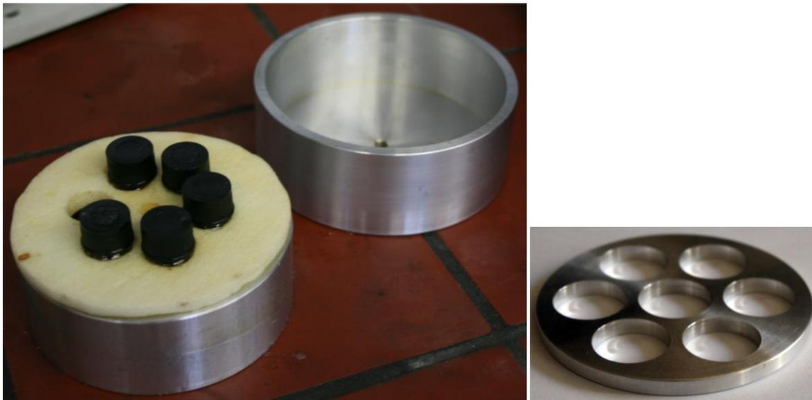
Fig. 18: The oil bath with sample vials and cover (left) and its inlet (right).
