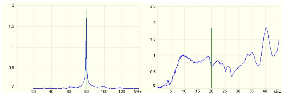
Fig. 17: Tuning curves of different cantilever. Left: soft cantilever for tapping mode (in dry environment). Right: cantilever in liquid for tapping mode in liquid.
