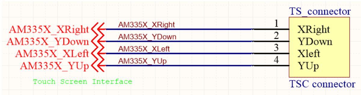
Figure 6.17: Schematics for the resistive touchscreen
