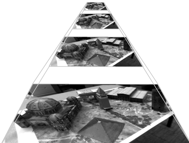
Figure 3.4: Schematic illustration of an image pyramid with four levels. Each level gets scaled down by scaling factor \alpha until a defined minimum size is reached. Tracking starts at the highest level and uses the current estimate as an initialization for the next level.
