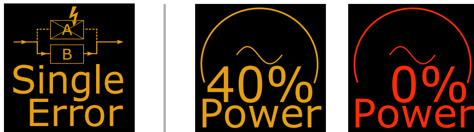
Figure 7.11: Proposed warning symbols displayed at the dashboard for driver information.
