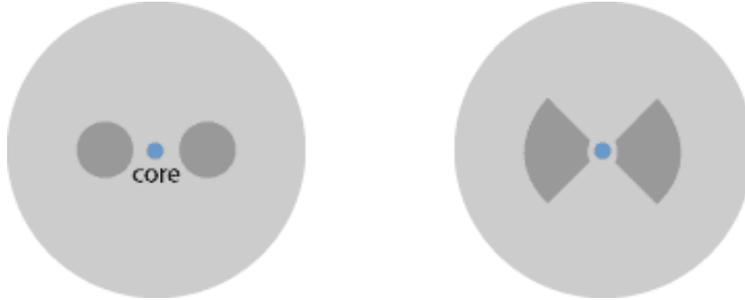
**Figure A.4:** Polarization-maintaining PANDA fiber (left) and bow-tie fiber (right). Introduced stress elements artificially increase the materials birefringence. Picture taken from [48].
