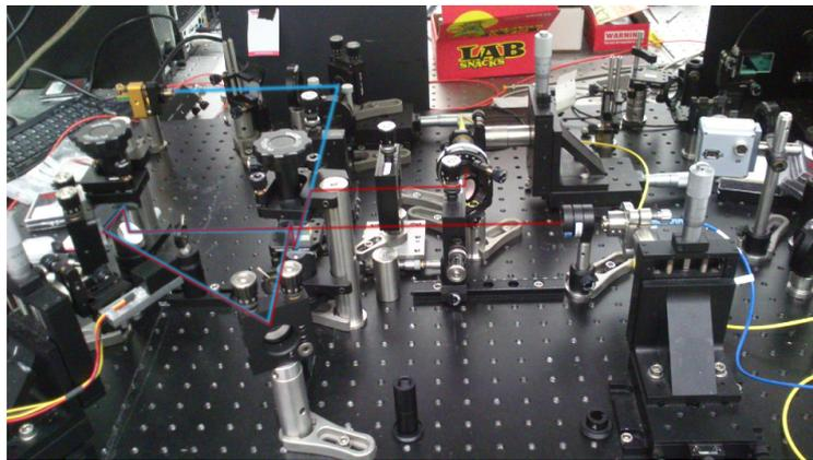
**Figure 5.2:** Photograph of the Sagnac loop setup. Instead of the usual HWP two periscopes were used to minimize beam aberrations and being able to also use the source for non-degenerate SPDC.
