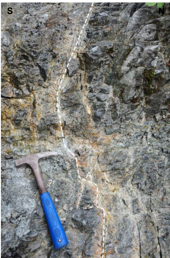
Fig. 38: West directing step joint. Dip direction and dip are 270/15 at N 47°23.049', E 014°30.352.
