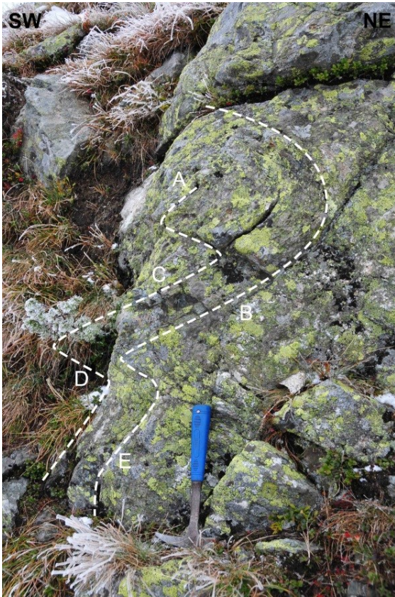
Fig. 37: Assumed disharmonic secondary z-fold. Dip direction and angle are: A = 230/25, B = 242/28, C = 242/30, D = 324/10, E = 212/45 at N 47°23.760', E 014°30.406'.
